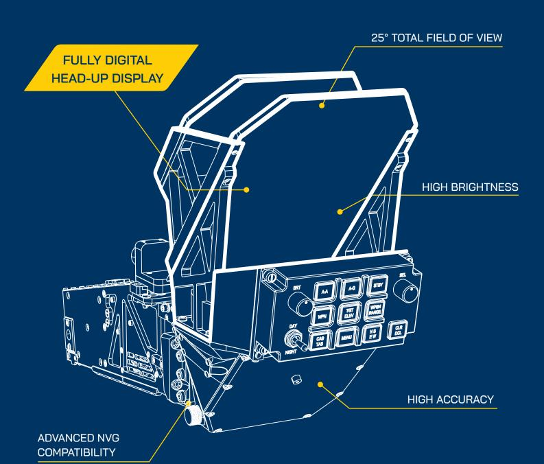
The PDU-159 is a fully digital, raster based and highly accurate "look through" display unit. The unit interfaces with the Mission Processor, MP-39 via a CAN bus for the unit control. For transferring video data - the displayed symbology, a HD-SDI link is routed between them. The PDU allows switching between day and night mode, the dual color backlight complies with any NVG (NVIS Class C, B, A).
