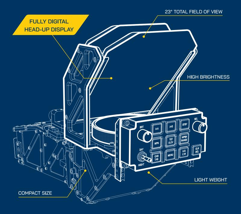
The PDU-39 is a fully digital, raster based, "look through" display unit. The unit interfaces with the Mission Processor, MP-39 via a CAN bus for the unit control. For transferring graphical data - the displayed symbology, a HD-SDI link is routed between them.
